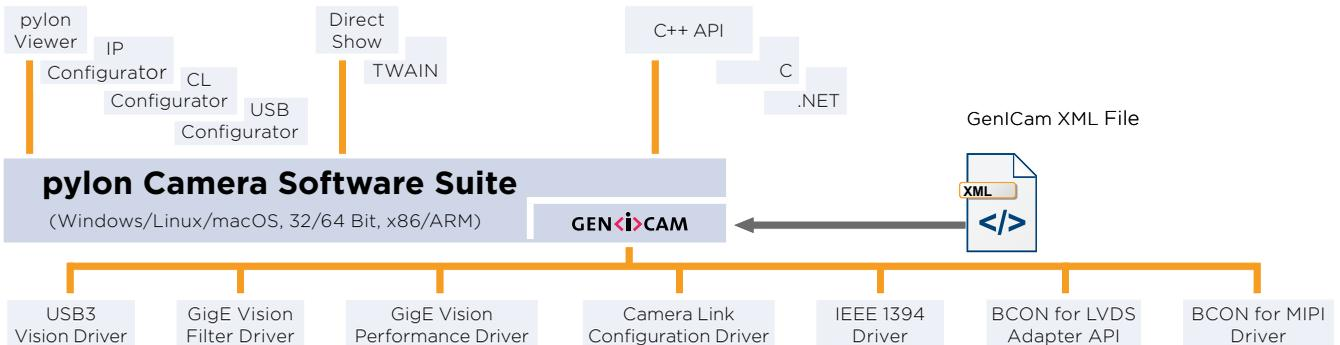
The architecture of the pylon Camera Software Suite is based on GenICam Technology, which offers you easy access to the newest camera models and the latest features. Changes to an existing camera device in your application essentially become a plug-and-play process.
